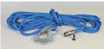
A-20-H1-SLT 20' of 5/16" AmSteel-Blue Synthetic rope w/H1 end hook (w/safety latch) installed on rope (RF included but not 100% installed)
