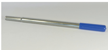
P7-3-EXT Safety Handle Extension for 3-ton unit. 18" long with blue grip. Inserts into P7-3.
