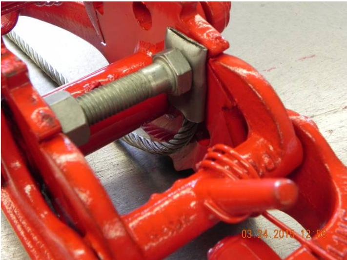
**Peen RF's rivet down with punch & ball peen hammer**
