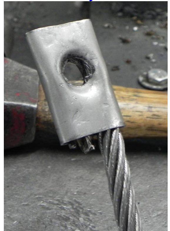
Hole is ready for rivet
